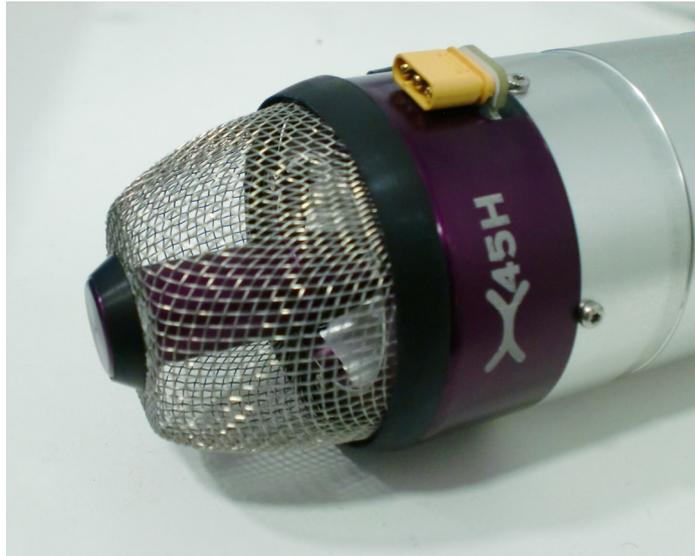
The supplied FOD screen is essential to protect the engine, USE IT!
