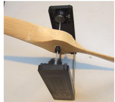
**Important - No attempt should be made to add material, lead shot or coloured sticky tape to balance the prop as this is sure to fly off later and if you are lucky it might not hurt someone, but the resulting out-of-balance running could cause major engine damage. If this happened in the air you would not know until it was too late. The warranty will not cover you for such damage.**
