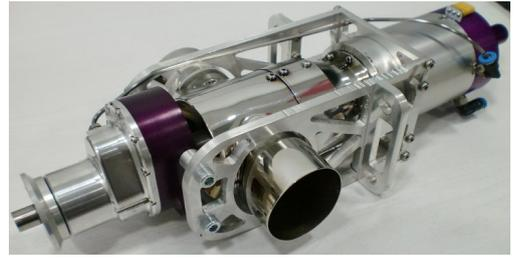
Use the special mounting supplied as part the engine. It provides critical support at the important positions required and aids heat dissipation from the small gearbox. It also gives the engine section gentle support and allows for expansion lengthways as the unit warms up in operation. It also provides some limited shielding from the hot interstage part between the engine and 2<sup>nd</sup> stage.
