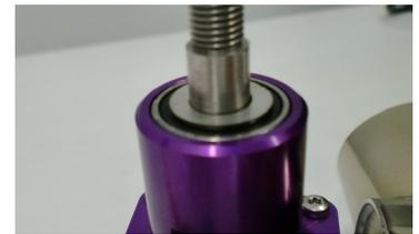
3. Place the 3/8" thin washer onto the output shaft first **before** the fan to ensure running clearance to the top bearing.
