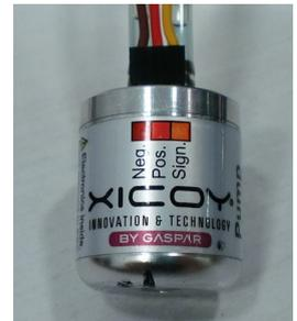
*Note: the three wires are NOT for the 3phases usually used for a brushless motor. The three wires are for the plus and minus power supply, and a single wire bidirectional digital link.*
